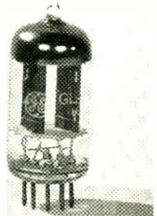
GL-5965 twin triode for computer use.
